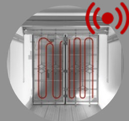
Loop cable inside the frame
